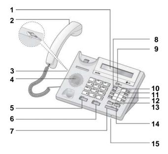
**LCD Display** 2 Handset 3 Headphone Socket (Ear/Mic Mode) Speaker 5 **Speaker Button** 6 Hold/Save Button 7 **Volume Button** 8 **Loop Button** Message Waiting LED 9 10 **Dnd/Fwd Button** 11 **Call Back Button** 12 Flexible Button 13 **Speed Button Trans/Pgm Button** 14 **Handsfree Microphone** 15
