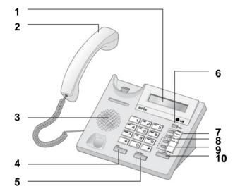
LCD Display (LDP-7004D only) **Handset** 3 **Speaker** 4 **OHD Button** 5 Hold/Save Button 6 **Message Waiting LED** 7 **Trans/Pgm Button** 8 **Speed Button** 9 Flexible Button 10 **Volume Button**
